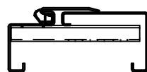
Befestigung Hutanker S2+TZ fissaggio staffa ad "U" S2+TZ fitting with "U" bracket S2+TZ
