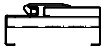
Befestigung Hutanker S2+TZ fissaggio staffa ad "U" S2+TZ fitting with "U" bracket S2+TZ
